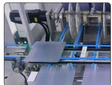
Photovoltaic industry, Stable detection of silicon wafers with very low reflectivity.
